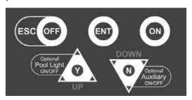
Each button is labelled with its primary function either on the button itself, or adjacent to it. Secondary functions are labelled within a curved white outline next to the relevant button.
