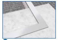
**5** Pour the concrete around the haunched drain base to the selected finished height required for your next step either tiling or finished concrete.
