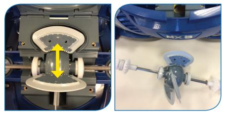
• Remove the engine and drive shaft assembly by holding both drive shafts and pulling firmly upward. Rotate the engine paddles if needed so that the engine can be easily removed.
