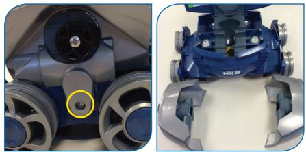
• Remove one screw from both left and right grey side body panels and remove both side panel assemblies.
