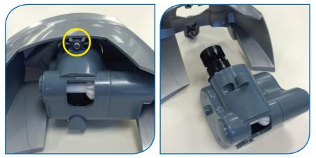
• Remove one screw and remove the reversing assembly from both side body assemblies.
