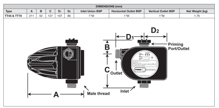
$<sup>^{\</sup>ast}$  Suction & delivery accept  $1^{1}\!/_{\!2}"$  PVC pipe on the I.D. and 2" fitting on the O.D.
