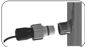
Figure 6. UV Sensor Installation
