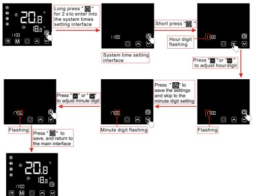
Notes: Under the clock setting interface, if there is no operation for 20 s, the system will automatically memorize use's settings, and return to the main interface; if short press 👿 'during any operating steps, the changes will not be saved and return to the main interface.
