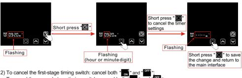
To cancel the second-stage timing switch: cancel both " <sub>ov2</sub> " and To cancel the two stage timing switch: cancel all " ov1"," <sup>ove1</sup>,", " over
