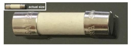
Fuse size is M205 (20mm x 5mm), TD6.5A (TD – Time Delay / slow-blow), HRC (High Rupture Capacity).
