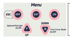
Each button is labelled with its primary function either on the button itself, or adjacent to it. Secondary functions are labelled within a curved white outline next to the relevant button. The buttons are backlit to show which are active at any given time, although the ESC/OFF button is always available to take you back to the home screen.
