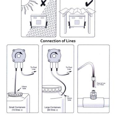
When inserting chlorine and acid tubes into dosing cell, tubes should penetrate approximately 50mm or half way into the depth of the mixing chamber. If the tube has a radius formed which is caused by the memory of the material, it is important that the tube point in the direction of the water flow.
