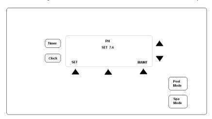
14. Press button located under the "MAINT" option and the following screen will be displayed;
