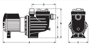
\*Suction and delivery accept 40mm PVC pipe on the I.D. and 50mm fitting on the O.D.
