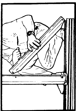
12. Connect diagonal brace (15) onto vertical and base channel using long bolts, spacer, nuts and washers (19). Fit skid member (18) to base channel (16) with bolt (20), nut (21) and washer (22).
