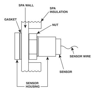
Figure 3 - Side view of installed sensor and housing
