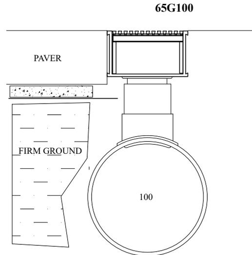
The Channel and Pavers should be laid on a bed of mortar.
