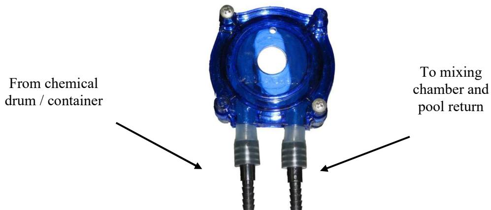
**Tip – to allow for easier fitting of tubes to pump barbs, soak end of clear supply hose in hot water for 30 seconds.**
